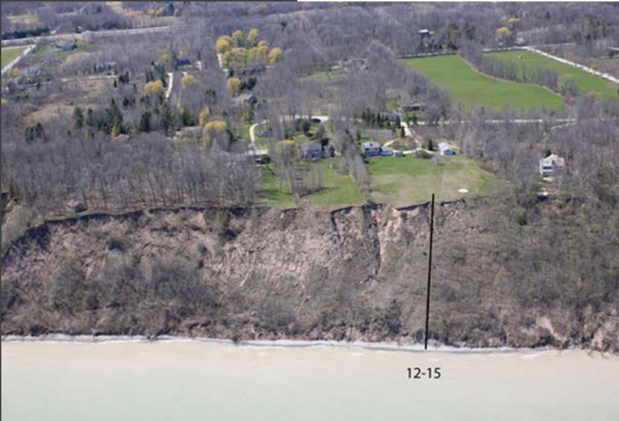
We measured 175 bluff profiles between Kenosha and Port Washington, Wisconsin, and they are in the process of being analyzed for lowest factor of safety which is a measure of how stable the bluff slope is. We tried to measure profiles at locations of profiles measured between 1976 and 1978 and again in 1995 but because the locations of these older
