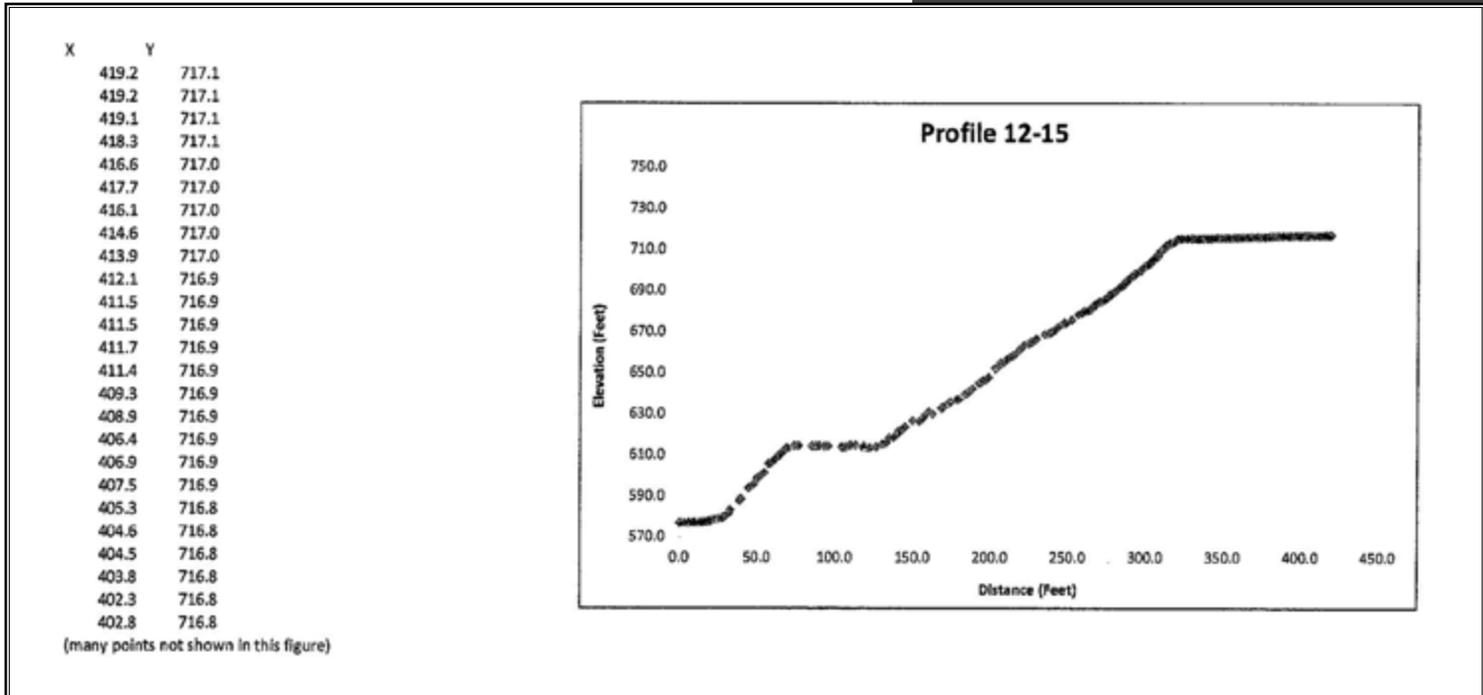
Figure 4 - Example of Excel file of bluff elevation and distances. The data column has been truncated. These files are used for the factor of safety calculations.
