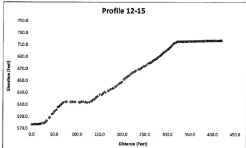
Figure 4 - Example of Excel file of bluff elevation and distances. The data column has been truncated. These files are used for the factor of safety calculations.
