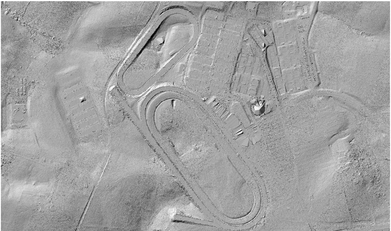
*Figure 5 - Hillshade example showing misclassifications in the ground surface*
