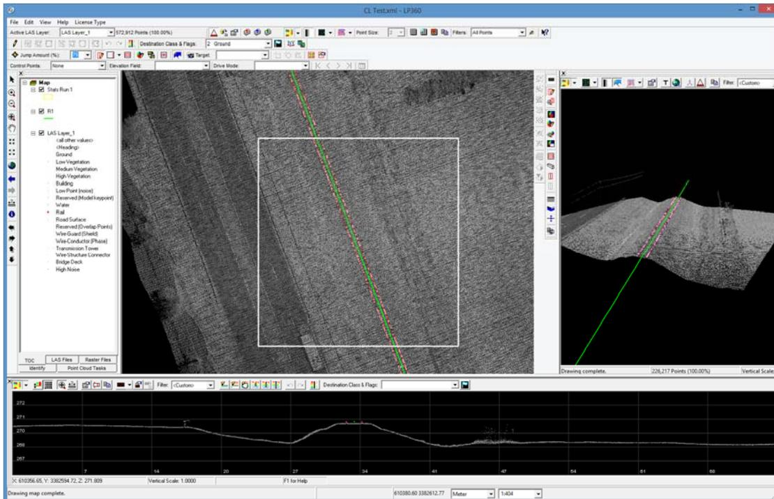
**Figure 1: A typical Alignment (green line), top of rail (red points) extraction**
